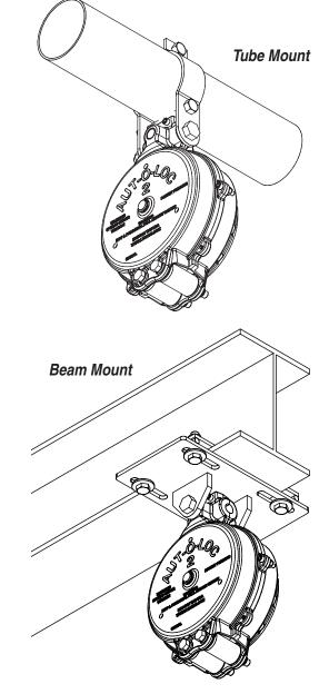
Tube and Beam Mounts can be mounted either parallel or perpendicular to the tube or beam. Tube Mount is shown perpendicular; Beam Mount is shown parallel.
