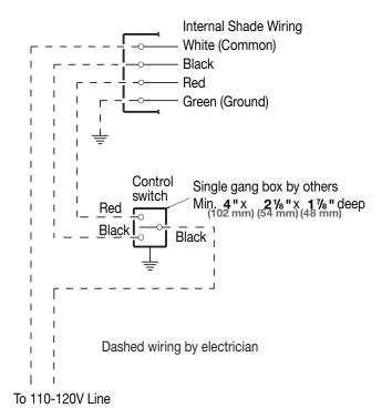
Please note: Test shade operation. If shade direction does not correspond with the switch orientation, turn power back off and switch the red and black wires from the motor to the switch.
