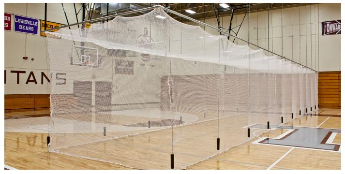
Just turn the key switch and the Bottom Lifting Practice Cage folds with no manual operation required. Lifting cables pass through d-rings on nylon belts with links attached to the netting that terminate at steel weights. A fully-automatic netting folds to the frame as the cage is lifted to a stored position. Features two corners with zippers for easy access.
