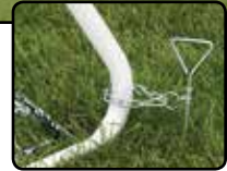
Auger-type ground anchors
