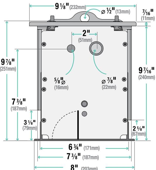
Standard Motor Wiring is on the AUDIENCE LEFT END of Screen Case.
